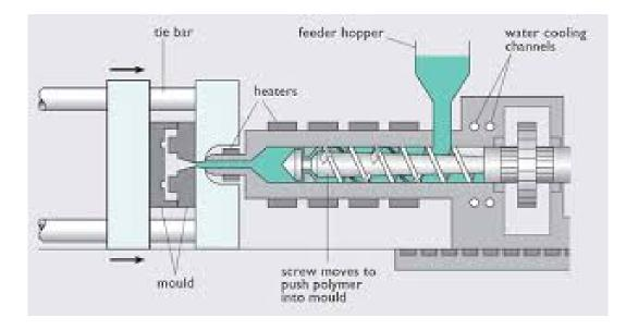
It is the most widely used cyclic process for product manufacture. This technique is widely used with thermoplastics. The process involves forcing or injecting the polymer into a closed mould where it takes the shape of the cavity.
