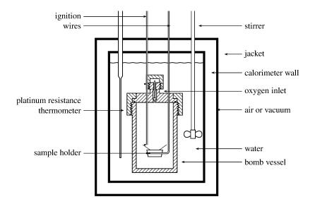
A weighed amount of food sample is placed inside the calorimeter, in a crucible. It is filled with oxygen under pressure. The calorimeter is immersed in a known quantity of water. The sample is ignited by means of electric fuse and heat liberated is measured by the rise in temperature.
